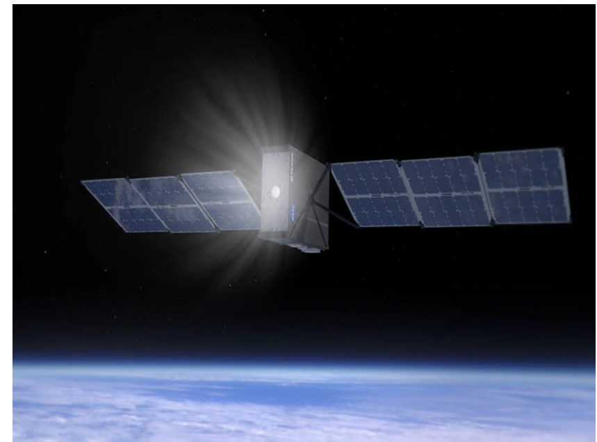
Courtesy: NASA Pathfinder Technology Demonstrator-1 spacecraft, demonstrating a water-based propulsion system in low-Earth orbit.
