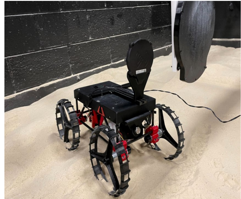
Courtesy: Astrobotic WPT for lunar rover
