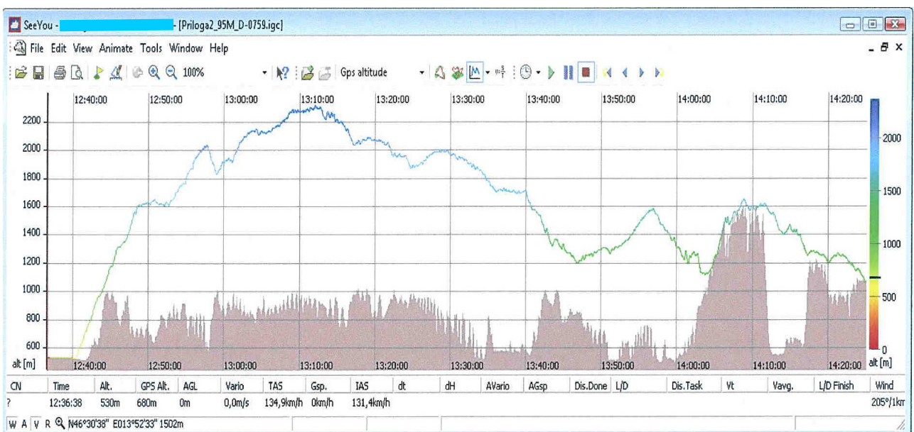
Image 2: Barogram of total flight, brown surface is presenting ground vertically under a plane
