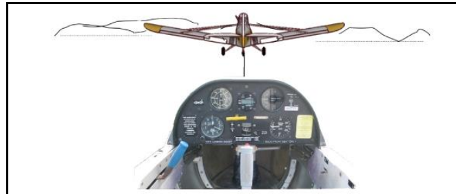
Figure 2: Visual Contact with the Towplane During Takeoff Phase
