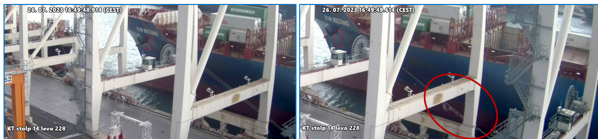
Figure 3: Situation at 16:49:51; breaking of the forward spring on the Xin Beijing (Source: VNC)
