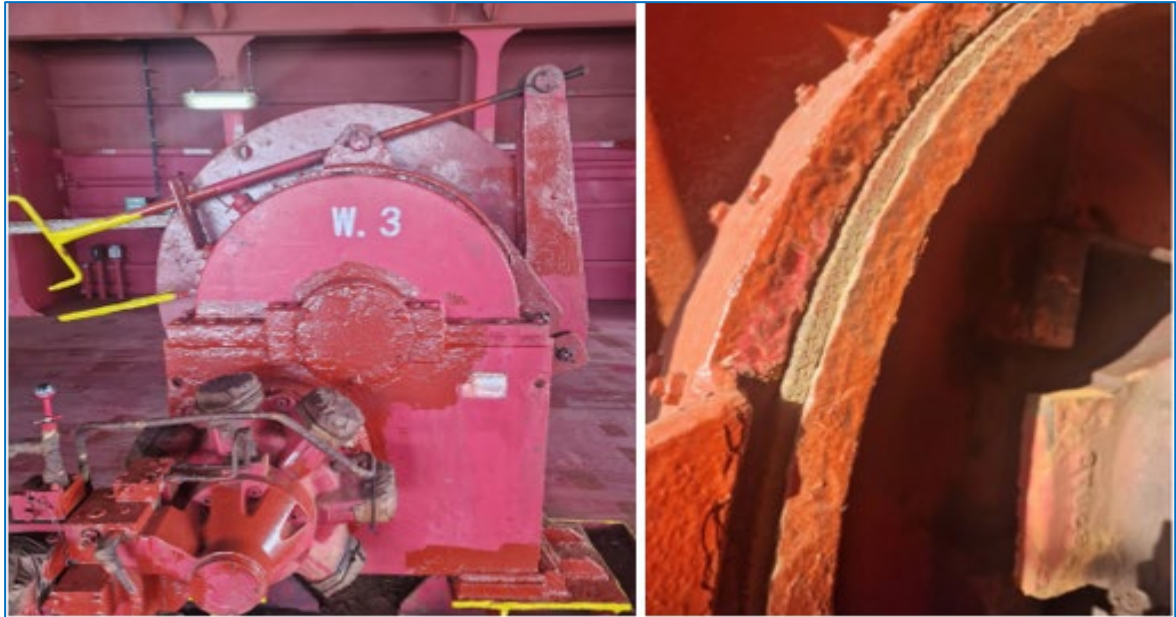
Figure 16: Stern winch and renewed brake linings (Sep. 2023)
