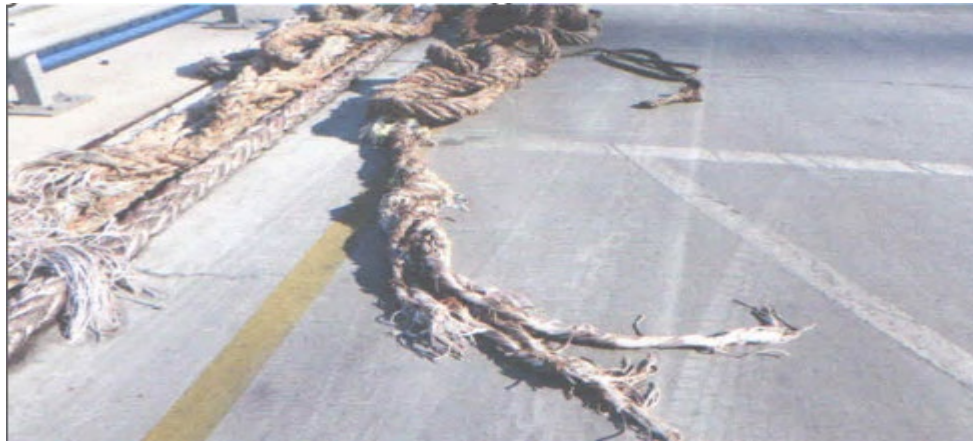
Figure 8: Damaged ropes, two types of ropes present
