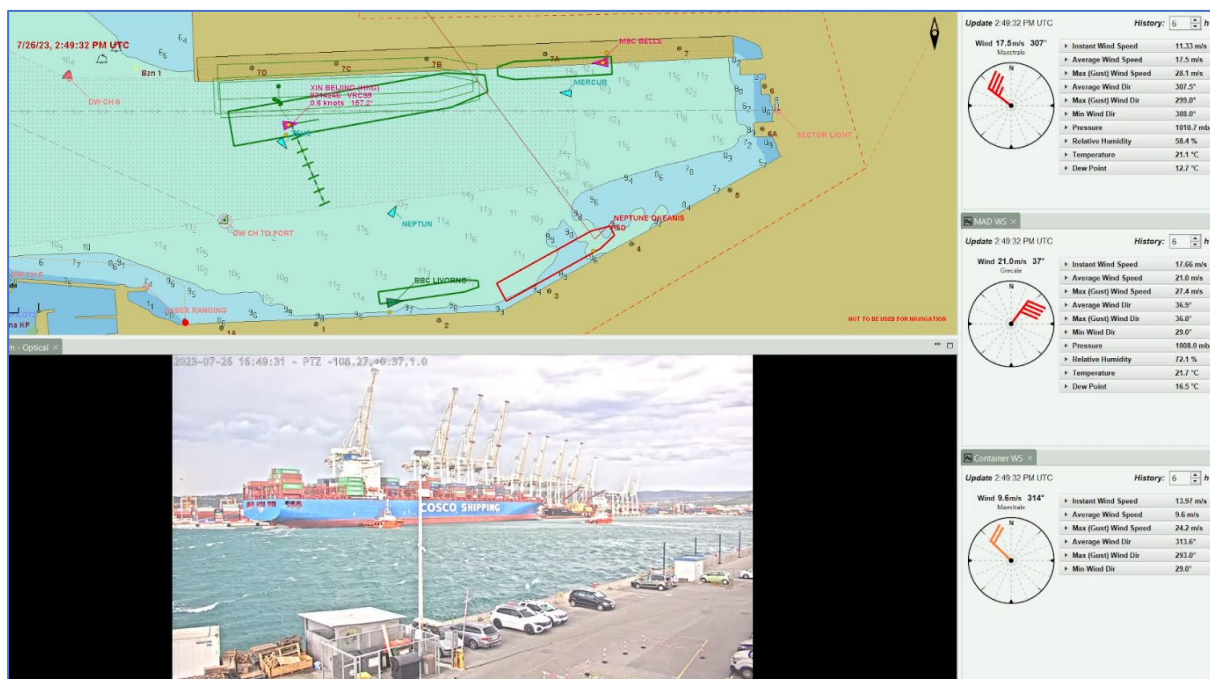
Figure 2: 16:49:32; Xin Beijing - aft springs breaking and stern lines slackening (Source: SMA)
