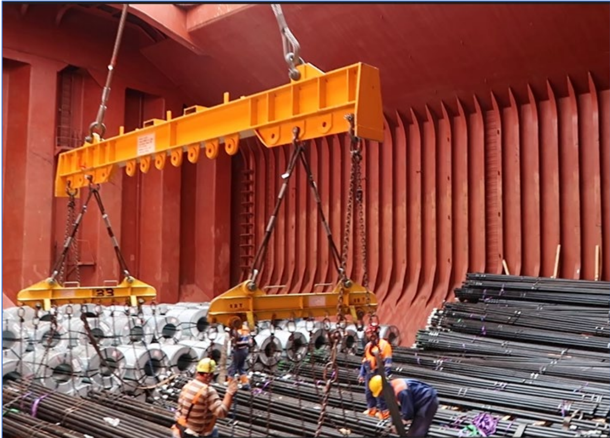
Figure 3: Pipes discharging using lifting beam
